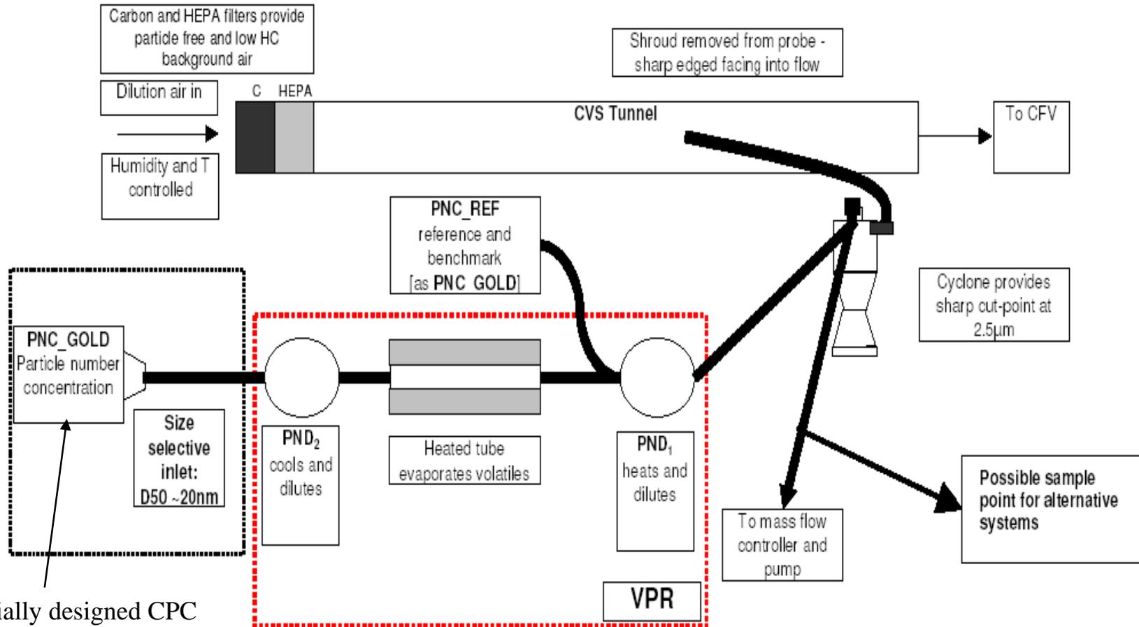
A specially designed CPC with a lower size cutoff of 23 nm is used
